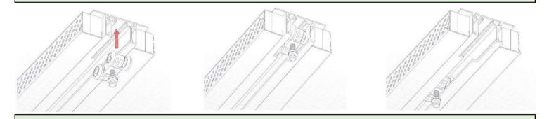
7. Hang the door, install stopper(or adjust soft close actuator) and cover plate
