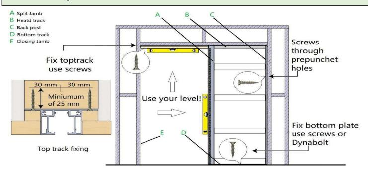
The **Head track** for all units must be fixed to the lintel at 300mm centres through the aluminium flanges on both sides of the track.
