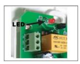
8.Power up the sensor and check whether the LED lights up.
