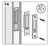
Insert striker plate assembly and secure with two No.8 1 screws.
