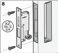
Insert the Privacy Lock assembly and secure with two No.8 3/4screws.
