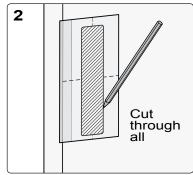
Wood Cutout: Remove middle section of flush pull template and mark cutout outline. Use midline as height reference. Mark for desired backset (35 or 50/55mm). Cut through all.
