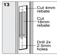
Place middle section of template into rebate and mark second rebate outline. Ensure it is the correct way up. Cut 18mm rebate
