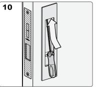
Use Mardeco hex tool to tighten grub screw inside top of flush pull. Ensure it is fitted firmly.
