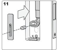
Insert spindle and emergency slide into the back of the lock slide. Choose the correct length spindle to suit your door thickness. Repeat steps 9 and 10 for installing the second flush pull.
