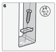
For wooden doors: install two woodfix brackets at top and bottom of cutout on both sides of the door.
