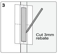
Remove middle section of end pull template and mark rebate outline on end of door. Use midline as height reference. Cut 3mm rebate.
