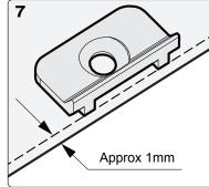
Fix brackets in centre of the cutout with the ridge facing outwards. Ensure that they are approx 1mm inside the edge and do not protrude.
