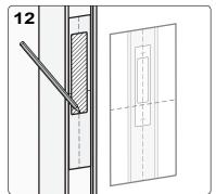
Remove middle section of striker plate template and mark outline for rebate. Use midline as height reference and ensure it lines up with the door. Cut a 4 mm rebate.
